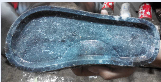
Figure 5: The real surface of slipper and result of the glue spread.
