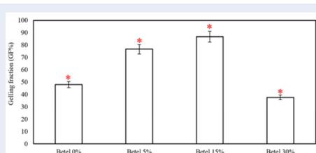
**Figure 15:** The gel fraction of the PVA/Chitosan/Gelatin hydrogels upon incorporating betel powder (\*p < 0.05)
