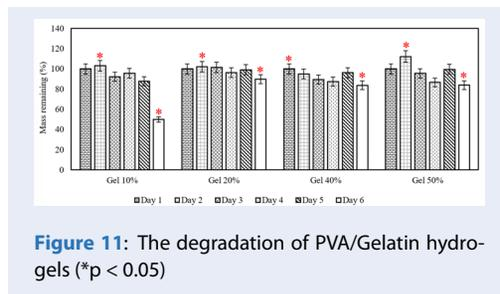
Figure 11: The degradation of PVA/Gelatin hydrogels (\*p < 0.05)
