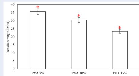
Figure 5: The tensile strength of the PVA hydrogels (\* $p < 0.05$ )
