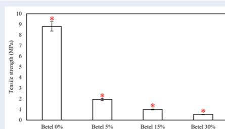
**Figure 17:** The tensile strength of the PVA/Chitosan/Gelatin hydrogels upon incorporating betel powder (\*p < 0.05)
