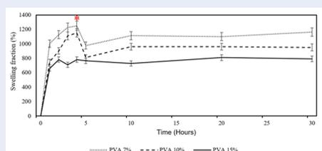
Figure 2: The swelling fraction of PVA hydrogels (\* $p < 0.05$ )
