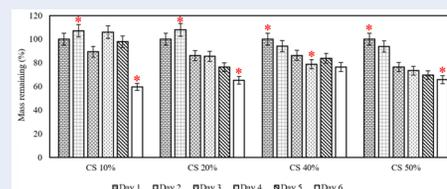
Figure 10: The degradation of PVA/Chitosan hydrogels (\*p < 0.05)
