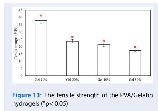
Figure 13: The tensile strength of the PVA/Gelatin hydrogels (\*p < 0.05)
