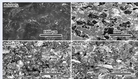
**Figure 18:** The surface morphology of the pure PVA/Chitosan/Gelatin hydrogel and the betel-added hydrogels with 5%, 15%, and 30% betel content.
