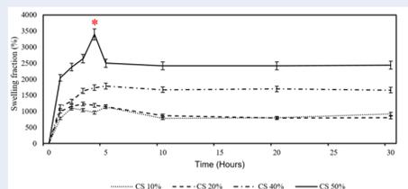
Figure 6: The swelling fraction of PVA/Chitosan hydrogels (\*p < 0.05)
