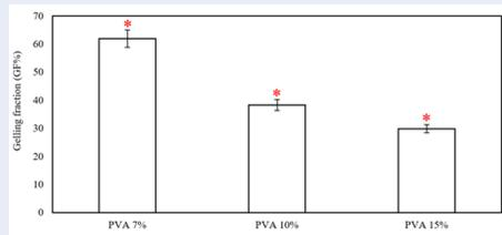
Figure 3: The gel fraction of PVA hydrogels (\* $p < 0.05$ )
