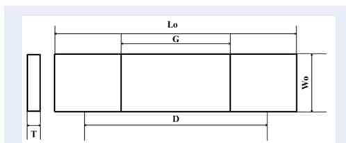
**Figure 1:** Illustration of hydrogel film following ASTM D882-18 standard
