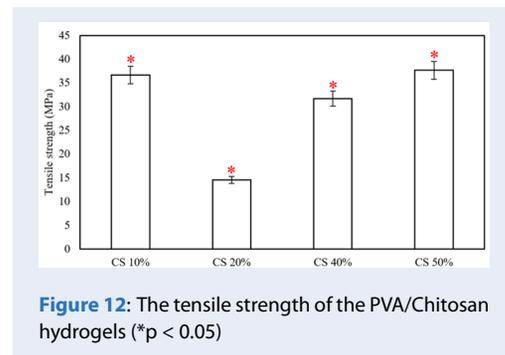
Figure 12: The tensile strength of the PVA/Chitosan hydrogels (\*p < 0.05)
