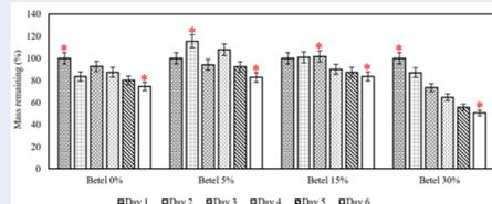
**Figure 16:** The degradation of the PVA/Chitosan/Gelatin hydrogels upon incorporating betel powder (\*p < 0.05)
