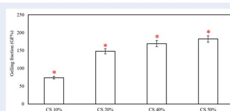
Figure 8: The gel fraction of PVA/Chitosan hydrogels (\*p < 0.05)
