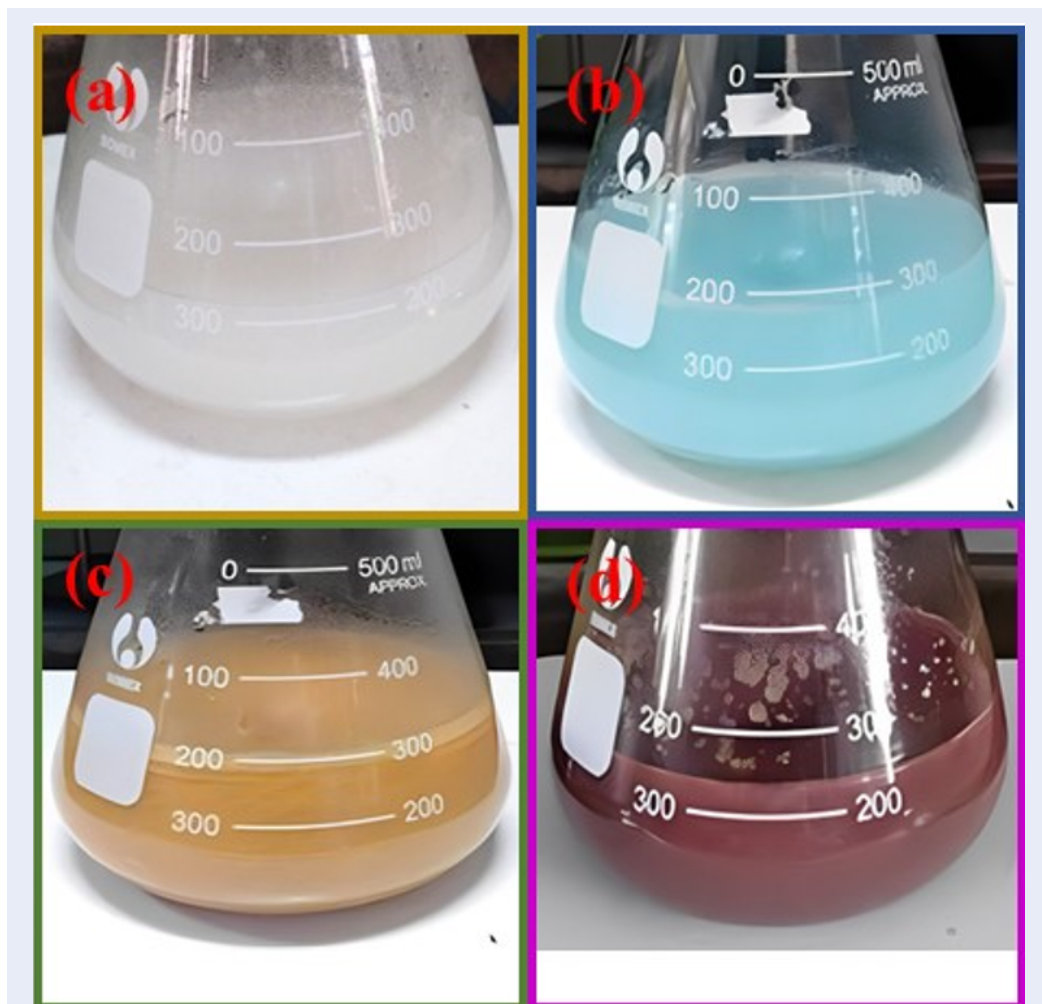
Figure 1: The BC suspension phase in water (a); after the addition of copper(II) acetate (b); after the addition of hydrazine for 1 min (c); after the addition of hydrazine for 14 h (d)
