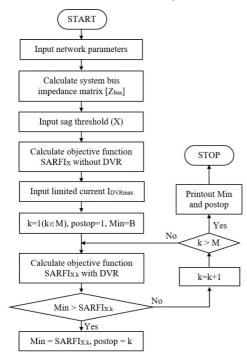
Fig. 4. Block-diagram of solving the problem of optimization
