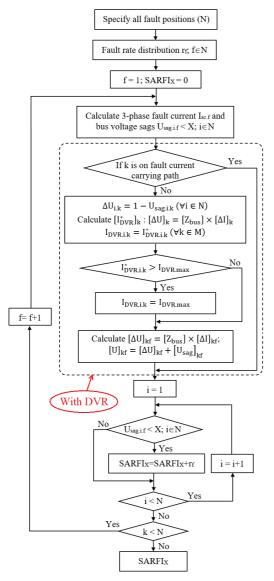
Fig. 5. Block-diagram of the part of SARFIX calculation without or with the presence of DVR
