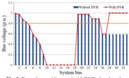
Fig. 8. Bus voltage without and with DVR placed on the branch 27 (27-28) for the short-circuit at bus 10
