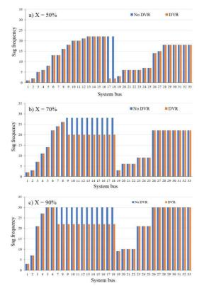
Fig. 14. Sag frequency at all buses for X=50, 70, 90% without or with DVR (at optimal placement),  $I_{DVRmax} = 0.3$  p.u
