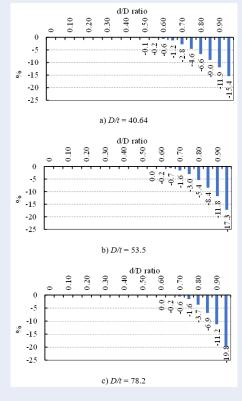
**Figure 7**: Reduction percentage of moment capacity of CFST sections with respect to *d/D*.
