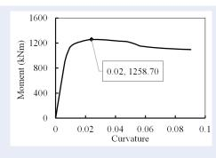
Figure 3: Moment–curvature curves of the CFST section
