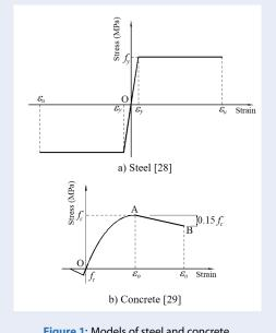
Figure 1: Models of steel and concrete.
