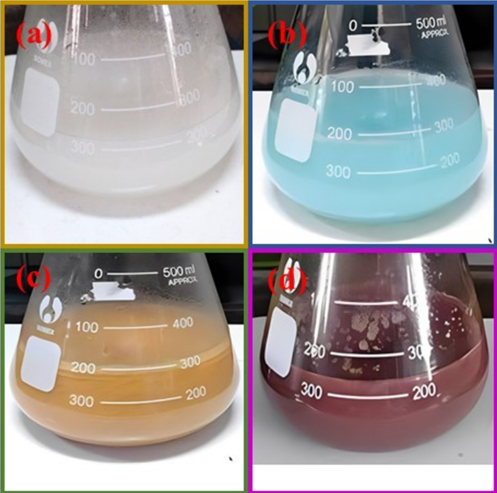
Figure 1: The BC suspension phase in water (a); after the addition of copper(II) acetate (b); after the addition of hydrazine for 1 min (c); after the addition of hydrazine for 14 h (d)
