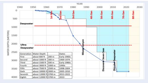
Figure 1: Evolution of operating water depths with different generations of floating drilling rigs
