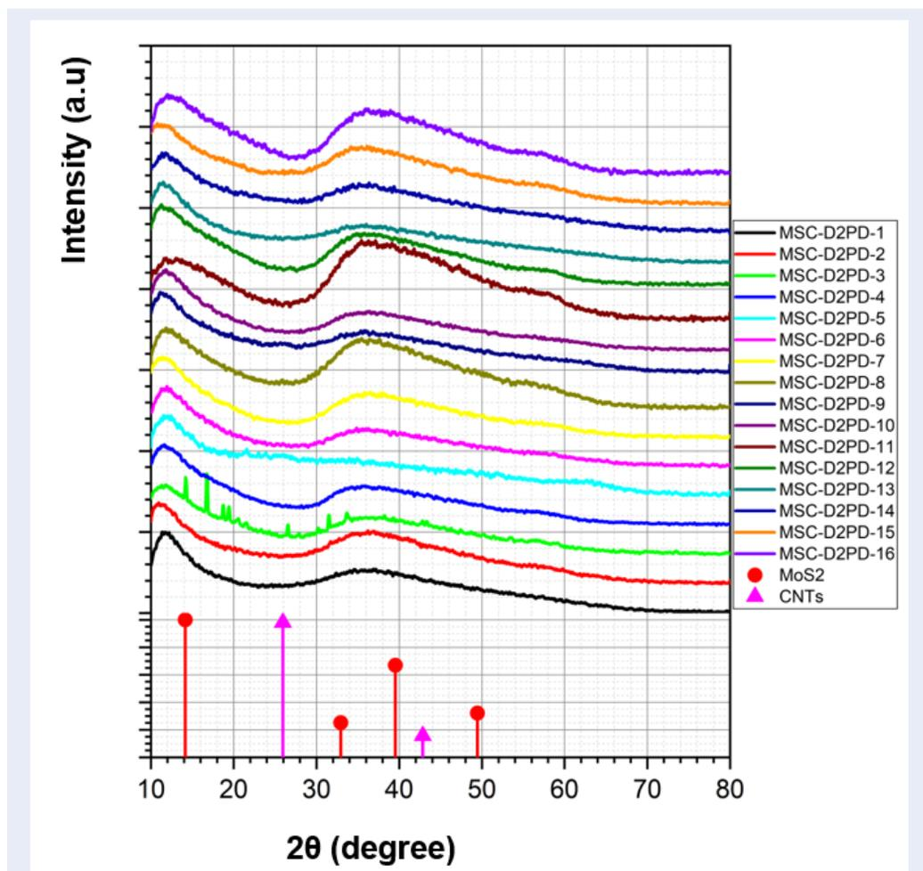
Figure 2: XRD patterns of 16 samples investigated from Taguchi method (Table 2)
