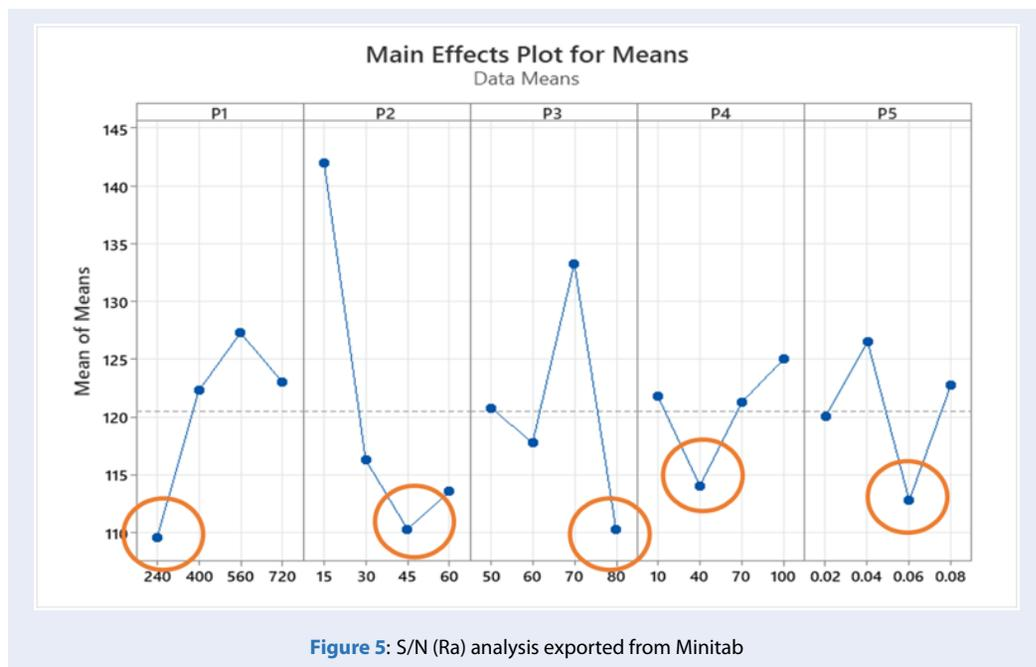
Figure 5: S/N (Ra) analysis exported from Minitab
