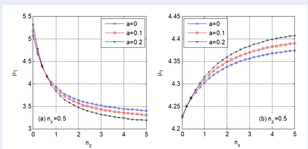
Figure 4: Variation of fundamental frequency parameters of (1-2-2) beam with the grading index for  $L/h=10$ ,  $\Delta T=20$  K and different porosity parameters
