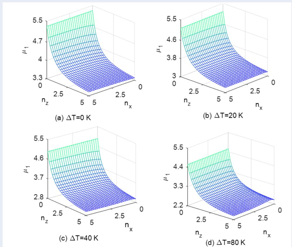
**Figure 2:** Variation of the first frequency parameter  $\mu_1$  of (1-2-2) beam with the power-law indexes for different temperature rise ( $L/h=20$ ,  $a=0.1$ )
