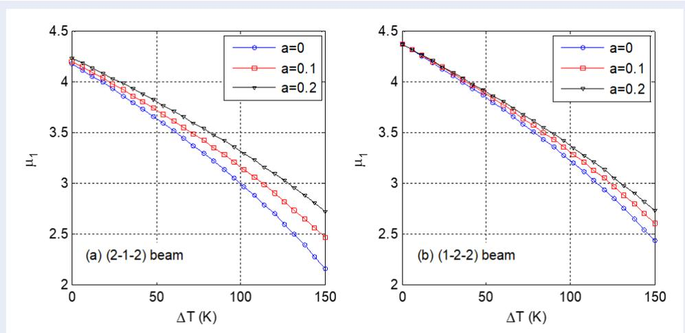
**Figure 6:** Variation of first frequency parameter with temperature rise for  $L/h=20$ ,  $n_x=n_z=0.5$  and different porosity parameters
