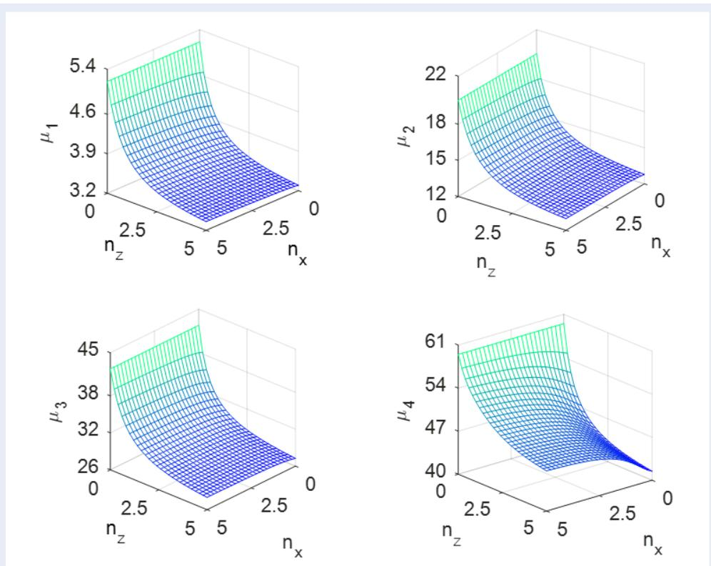
Figure 3: Variation of the first four frequency parameters of (1-2-2) beam with the power-law indexes for  $L/h=10$ ,  $a=0.1$ ,  $\Delta T=20$  K
