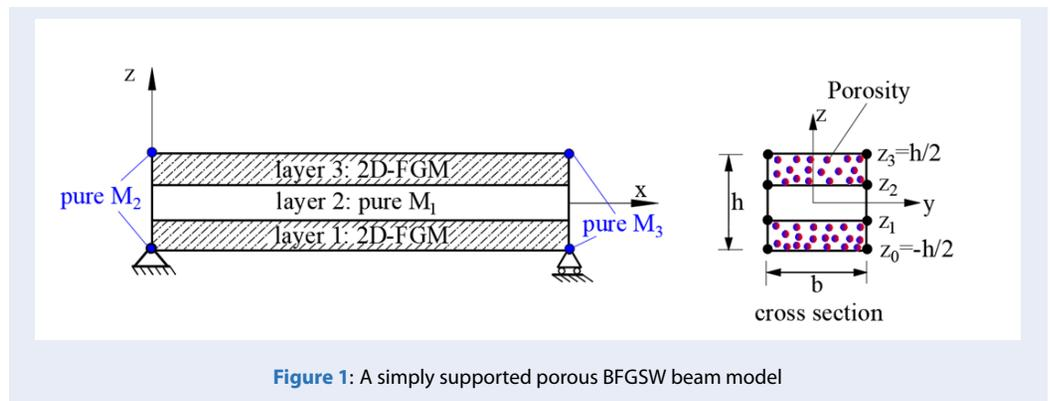
Figure 1: A simply supported porous BFGSW beam model
