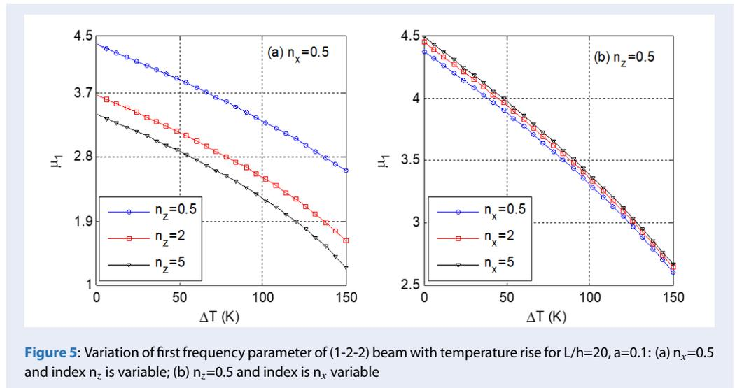
**Figure 5:** Variation of first frequency parameter of (1-2-2) beam with temperature rise for  $L/h=20, a=0.1$ : (a)  $n_x=0.5$  and index  $n_z$  is variable; (b)  $n_z=0.5$  and index is  $n_x$  variable
