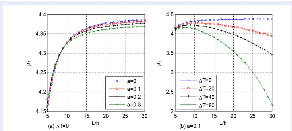
**Figure 7:** Variation of first frequency parameter of (1-2-2) beam with length-to-height ratio  $L/h$  for  $n_x=n_z=0.5$ : (a)  $\Delta T=0$  and different porosity parameters; (b)  $a=0.1$  and different temperature rises
